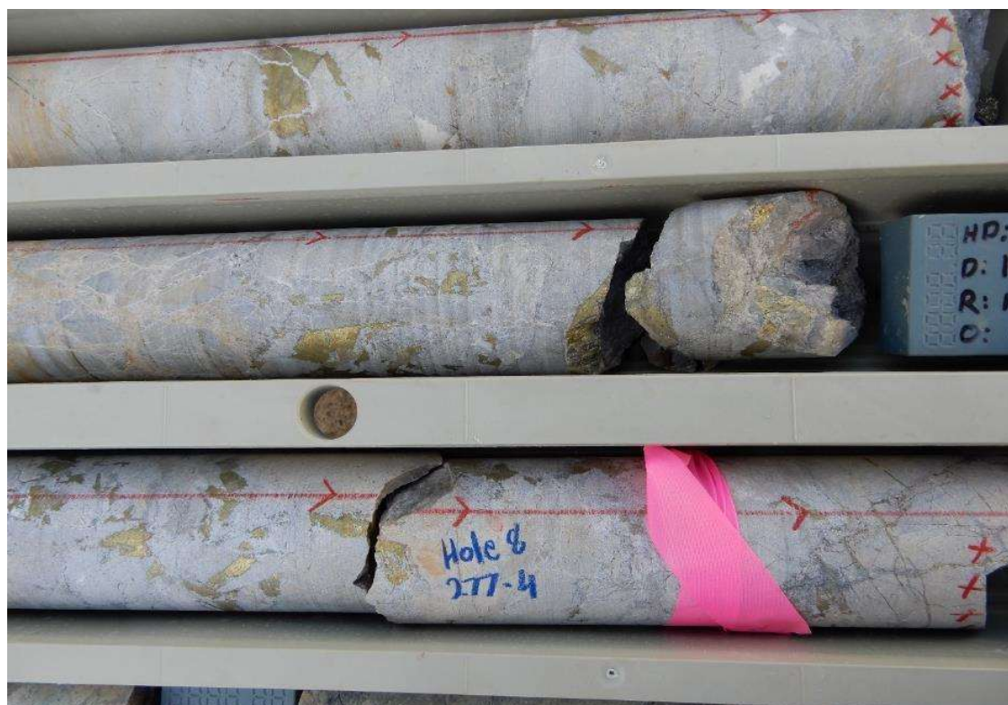
Fig 9 HQ Core photo hole 21CAEDD008, 275m-277m. Chalcopyrite rich infill in clast supported hornfels breccia. Primary zone 275m-277m assays 2m @ 1.69% Cu, 0.23 g/t Au, 16.8 g/t Ag, 3.22 % S.
