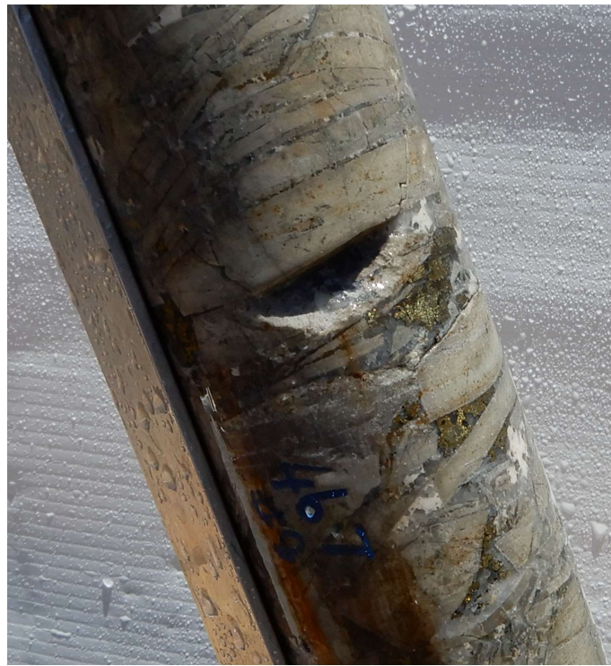
Fig 10 HQ Core photo hole 21CAEDD007, 445.8m. chalcopyrite rich infill in clast supported hornfels diorite breccia. Primary zone 445m-446m assays 1m @ 0.99% Cu, 0.2 g/t Au, 23.5 g/t Ag .
