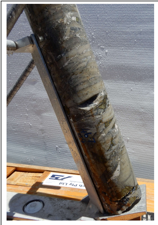
Fig 10 HQ Core photo hole 21CAEDD007, 445.8m. chalcopyrite rich infill in clast supported hornfels diorite breccia. Primary zone 445m-446m assays 1m @ 0.99% Cu, 0.2 g/t Au, 23.5 g/t Ag .
