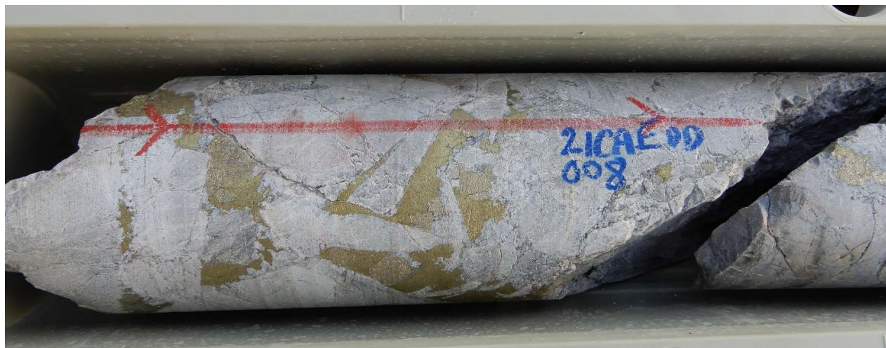
Fig 8 HQ Core photo hole 21CAEDD008, 218.5m. Chalcopyrite rich infill in clast supported hornfels breccia. Primary zone 218m-219m assays 1m @ 2.18% Cu, 0.38 g/t Au, 21 g/t Ag, 4.71 % S.
