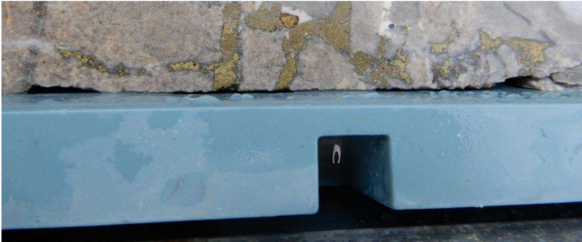
Fig 10 HQ Core photo hole 21CAEDD007, 445.8m. chalcopyrite rich infill in clast supported hornfels diorite breccia. Primary zone 445m-446m assays 1m @ 0.99% Cu, 0.2 g/t Au, 23.5 g/t Ag .
