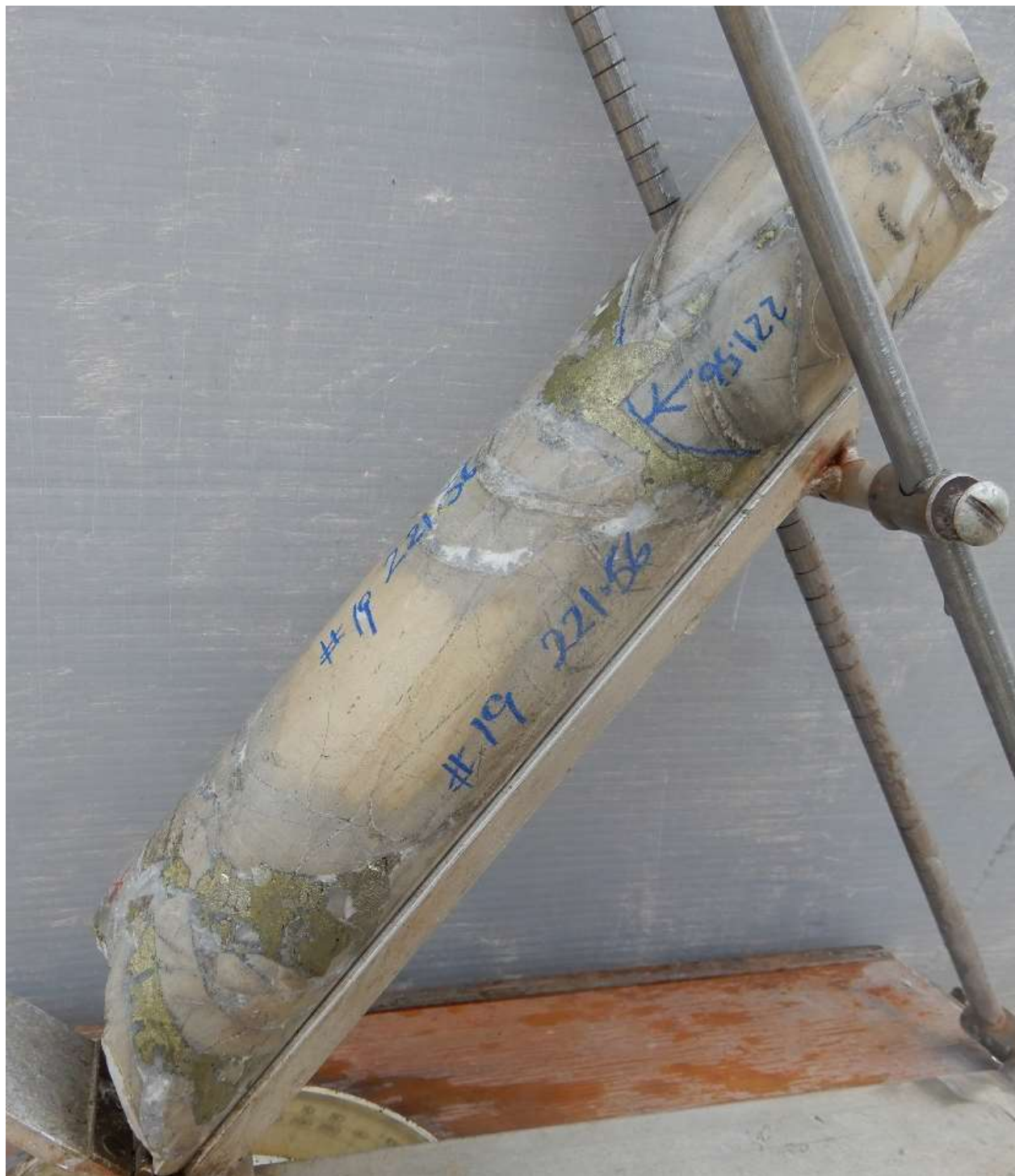
Fig 12. Photo full HQ core Hole #19, oriented in core oriented frame, hole drilling to south south west , view looking west north west , hole at 221m inclined at -51 degrees toward 218 degrees mag: Hydrothermal Infill Breccia. Clasts dominated by yellow grey, sericite altered hornfels, with infill of chalcopyrite (golden) , pyrite (brassy) ,minor calcite (white) ,quartz (glassy).
