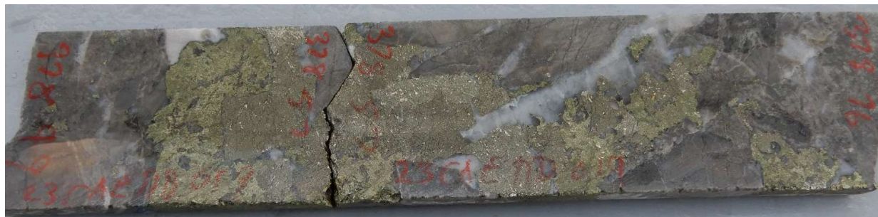
Infill in hydrothermal breccia of high grade chalcopyrite (golden) with well formed pyrite (brassy), some quartz (light grey) and calcite in a breccia dominated by angular clasts of yellow grey hornfels. CAE Hole 19, 378.5m. 1m interval 378m-379m : 1.90% Cu, 0.66 g/t Au, 83.7 g/t Ag, 6.45% S.
