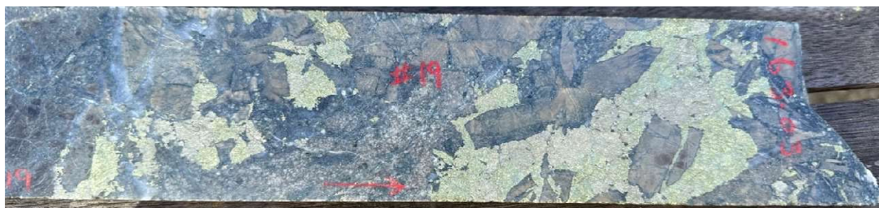
Infill in hydrothermal breccia of high grade chalcopyrite (golden) with well-formed pyrite (brassy), some quartz (light grey) in a breccia dominated by angular clasts of yellow grey hornfels, some altered porphyry. CAE Hole 19, 163m. 2m interval 162m-164m : 1.64% Cu, 0.39 g/t Au, 20.3 g/t Ag, 6.15% S.
