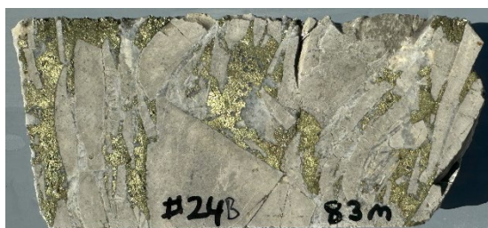
High grade chalcopryrite infill in hornfels breccia. CAE Hole 24, 83m . 2m interval 82m-84m : 3.04% Cu, 0.23 g/t Au, 102.9 g/t Ag, 4.11% S (2m @ 4.0% CuEq).
