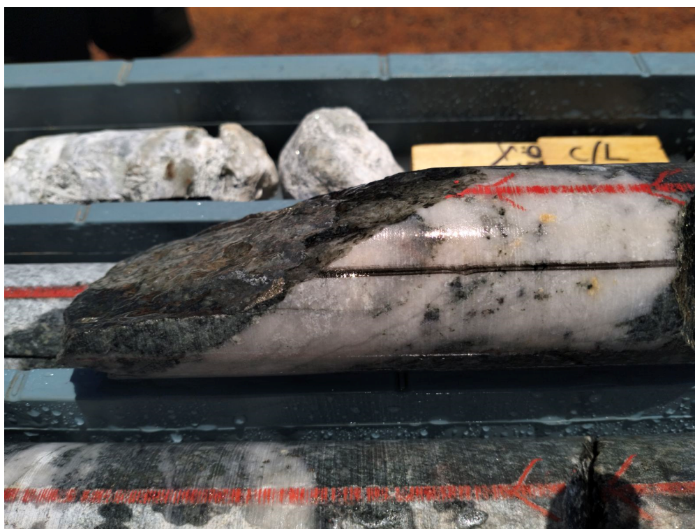
Figure 6, Orientated diamond core with mineralisation in quartz veining
