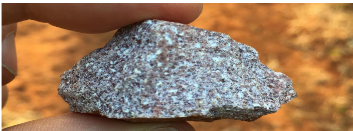
Figure 2: A rock chip sample showing high levels of gibbsite-hosted Al 2 O 3 from a previously untested area.
