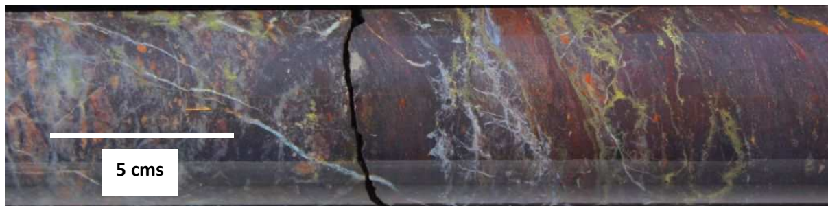
Figure 3d: Diamond drill hole APDD002 core photo from 65.20 to 65.40 metres showing carbonate veinlets (white) and stringer sulphides (chalcopyrite – pyrite) (yellow) within strong haematite alteration (red – brown).
