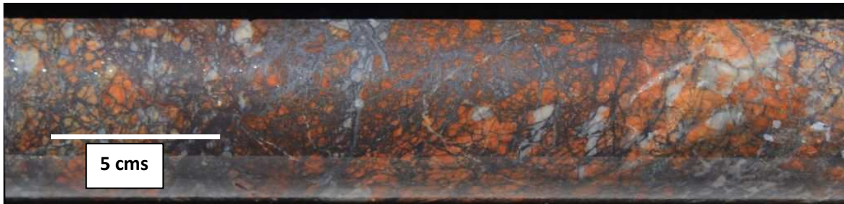
Figure 3b: Diamond drill hole APDD002 core photo from 42.00 to 42.20 metres down hole showing brecciated granite and strong haematite – chlorite – red rock alteration.
