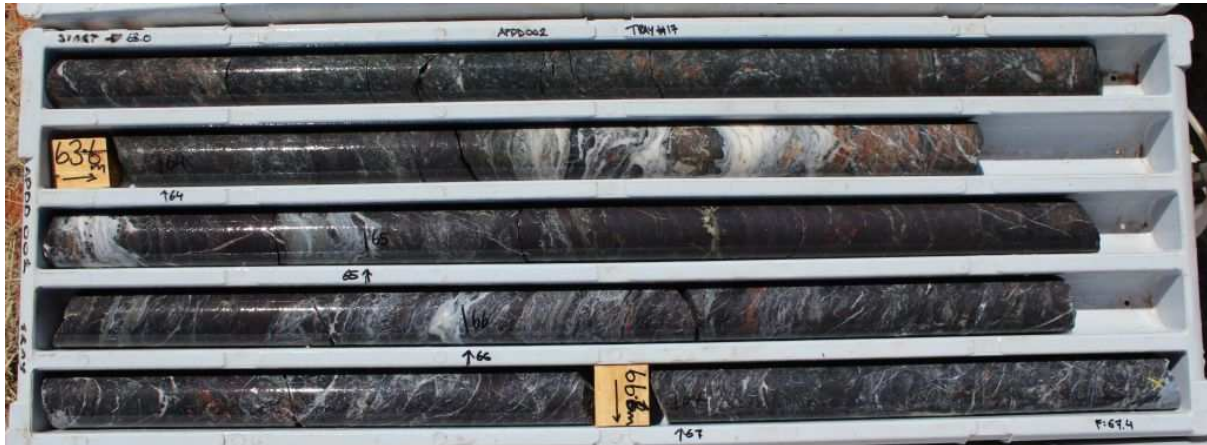
Figure 3c: Diamond drill hole APDD002 core photo from 63.00 to 67.40 metres down hole showing quartz – haematite – fluorite alteration and stringer sulphides (chalcopyrite – pyrite).
