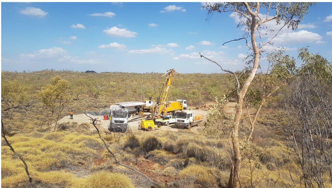
Figure 1: DDH1 diamond rig and support gear on FNDD001 drill site
