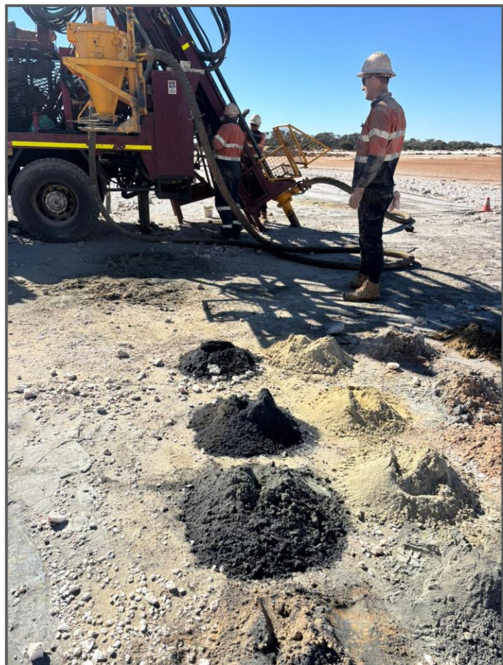
Figure 1. Aircore drilling commences at Goongarrie.
