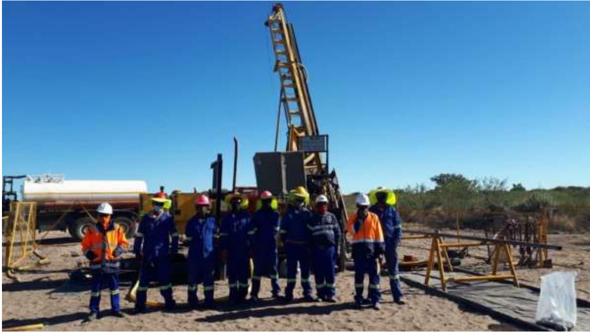
Figure 3. DC rig drilling the first stratigraphic hole into the Perseverance Prospect.
