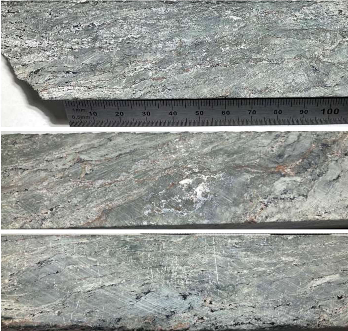
Figure 1. High-grade chalcocite (silver-black metallic mineral) from drill hole NCP20A. The displayed drill core is grading at 10.9% Cu and 45 g/t Ag. This zone marks the base of the mineralised section and extends for 1.7m downhole.
