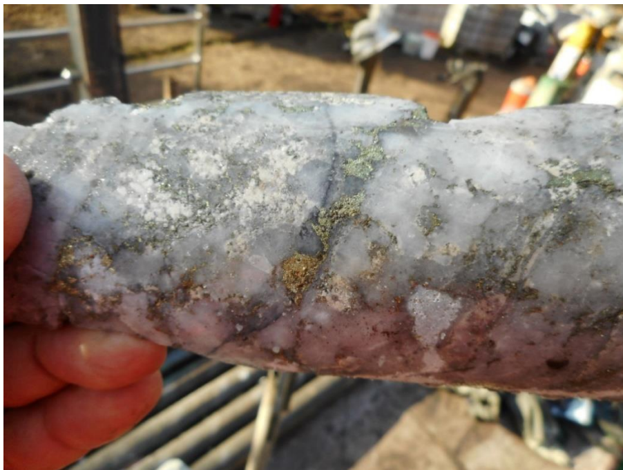
Figure 5 Mineralised Quartz Zone - BD019-003
