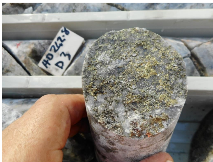
Figure 6 Chalcopyrite on Fractures in Quartz Zone - BD019-003
