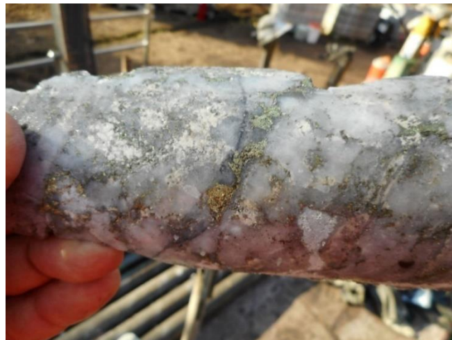
Massive quartz interval in BD019-003 28m at 0.83% Cu in the “out-flow” zone
