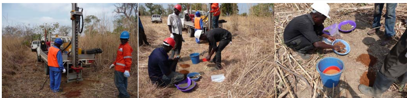
Auger drilling, sampling and logging at the South Wa soil anomaly – January 2011
