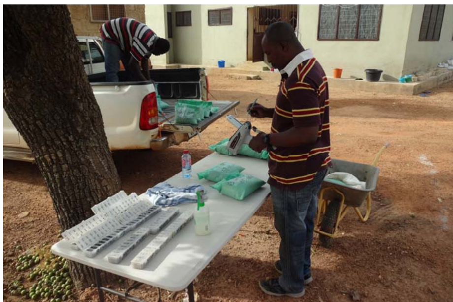
Hand held XRF analysis of RC drill chips at Wa Exploration house in NW Ghana
