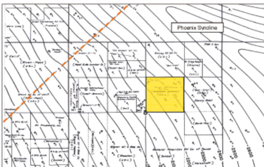
Figure 2. Wellington-Maricopa lease shaded yellow on southwest flank of Phoenix syncline in SW/4 of NE/4 of Section 8. Dashed orange line shows location of cross-section K-L in Figure 3. Modified after CDOG, 1985
