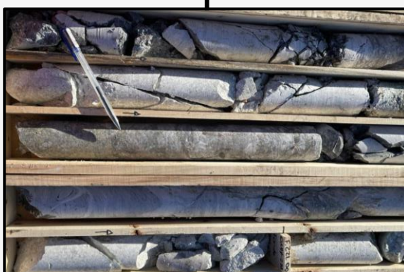
GNDD-288 Magnata Fault (217-220m)
