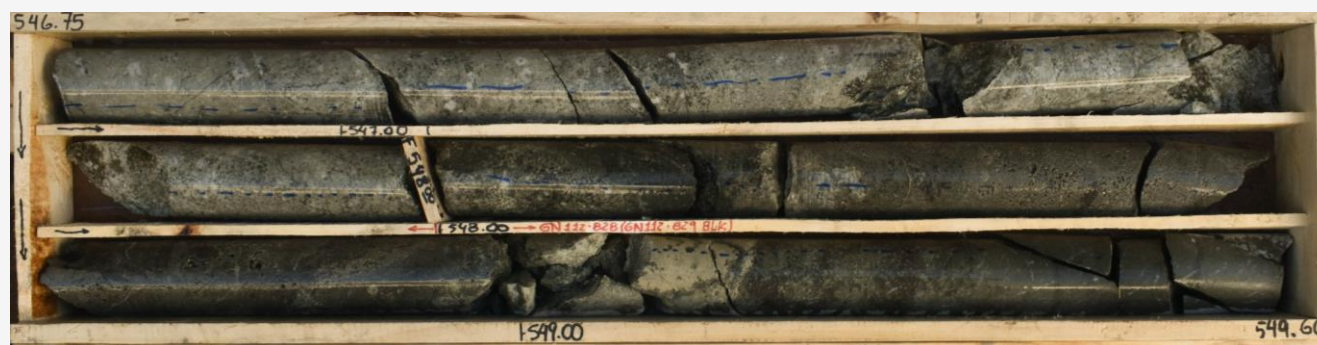
GNDD-685 (547.0-549.3m) : massive sulphides (50% Pyrite, 30% Sphalerite) 100 metres below MRE boundary
