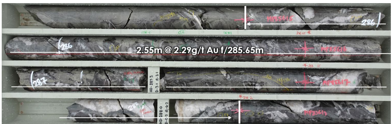
Figure 12. Quartz veining within PHD001 (285.1m to 288.5m shown).
