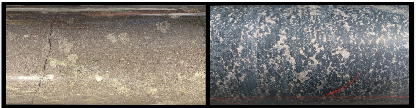
Figure 6. Typical sulphide mineralisation intersected in JD002: hypogene massive sulphides comprising pyrrhotite-pentlandite-chalcopyrite at ~49.5m down-hole (left) and matrix/net textured pyrrhotite-pentlandite-chalcopyrite at ~90.5m down-hole (right).
