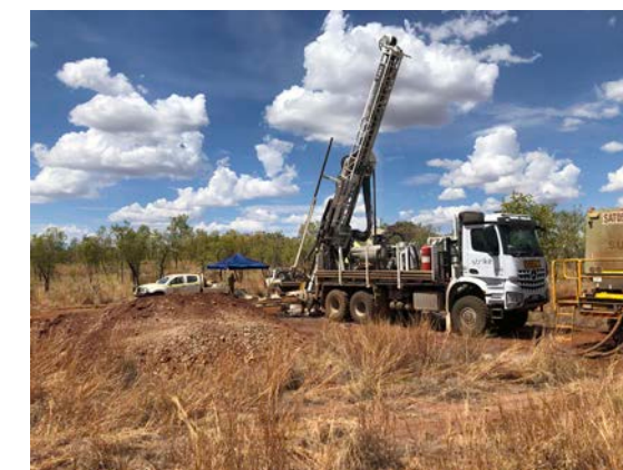
Figure 12: RC Drilling at the Hawkstone Project, WA.
