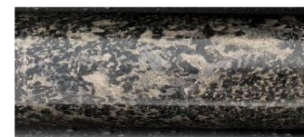
High-sulphide, base metal-rich mineralised zones Up to 11g/t 3E, 2% Ni, 1% Cu
