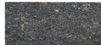
Low-sulphide disseminated mineralisation between HG zones 0.6-0.8g/t 3E, ~0.15% Ni, ~0.08% Cu
