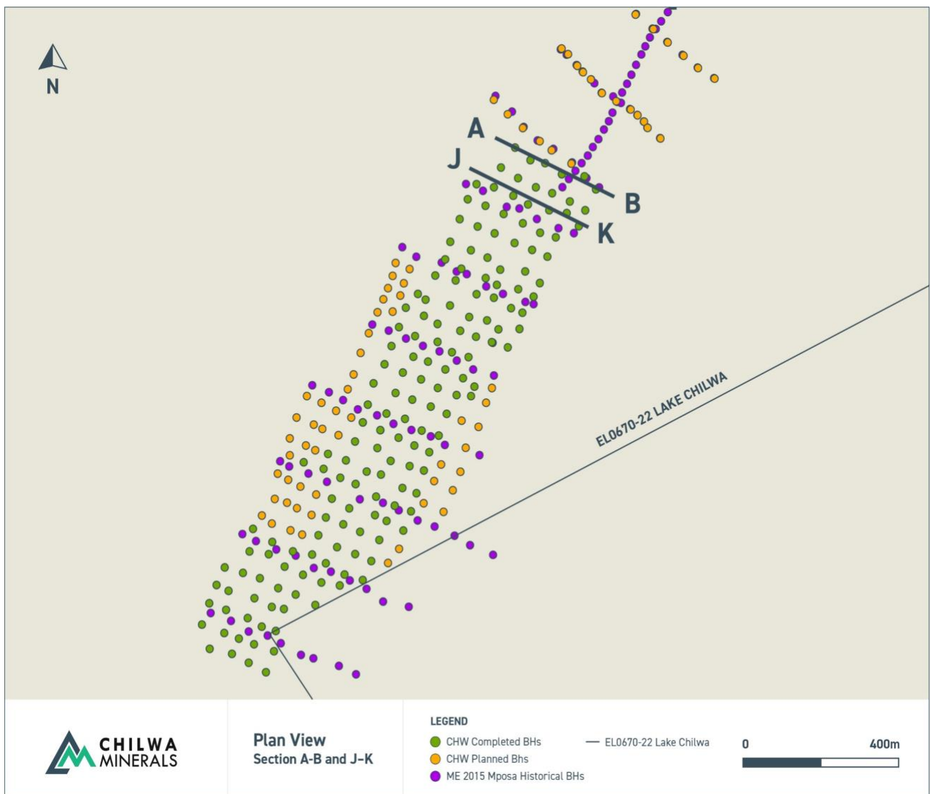
Figure 2 – Mposa Drilling Program Showing Drill Collar Locations for Assay results received or currently being analysed (green)
