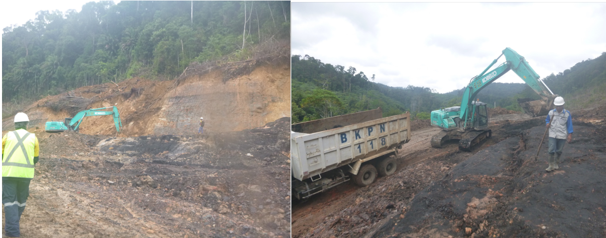
OB Removal and coal cleaning at BBM-Anak Project
