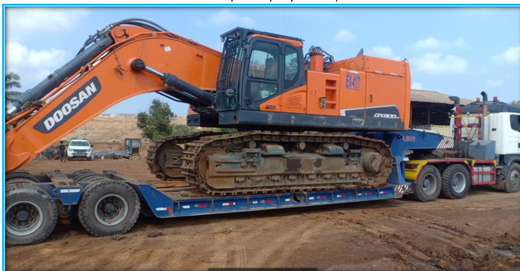
80t class excavator (Doosan 800) on progress mobilisation
