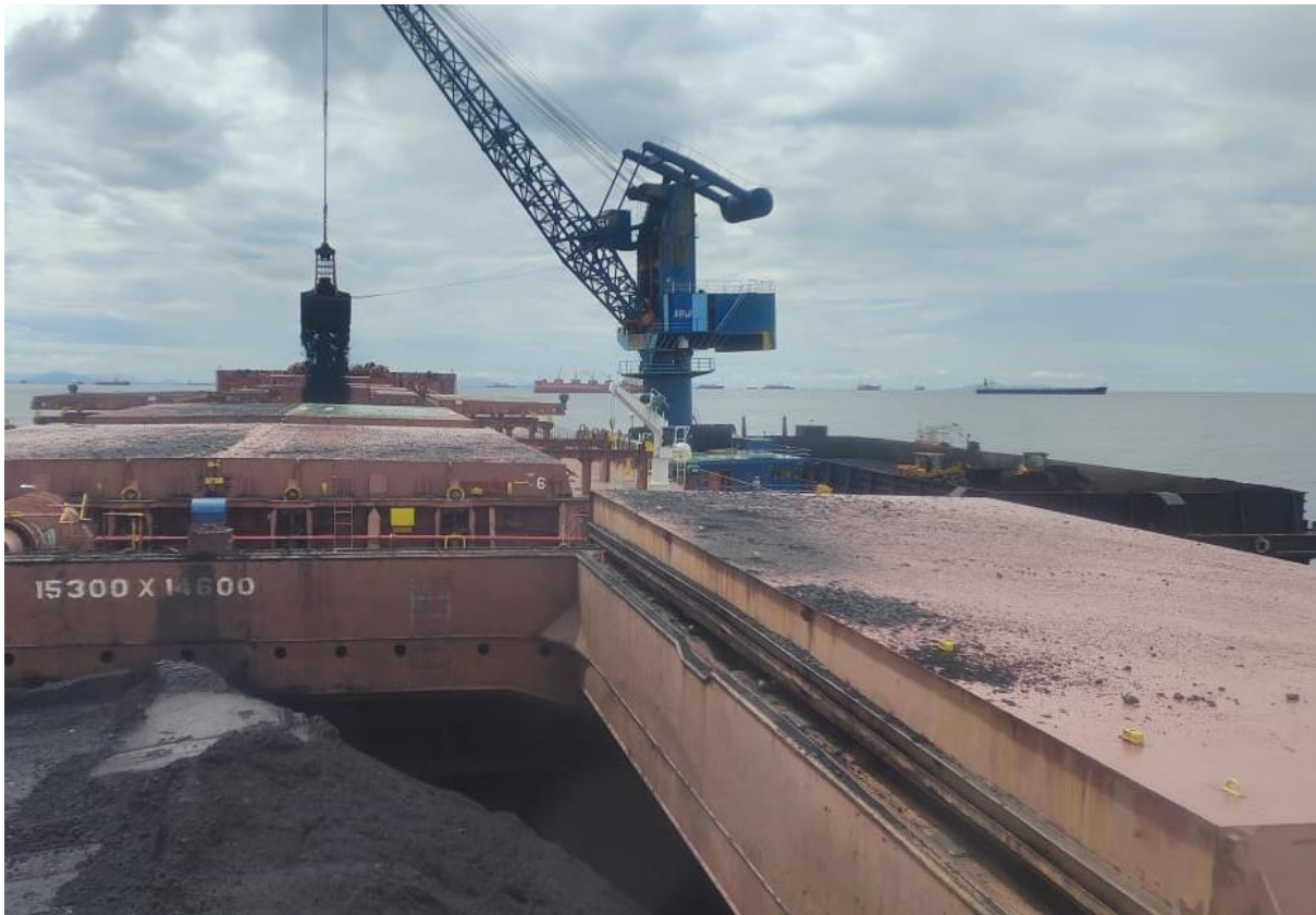
Crane at-sea-loading of coal from Cokal's barge to the vessel
