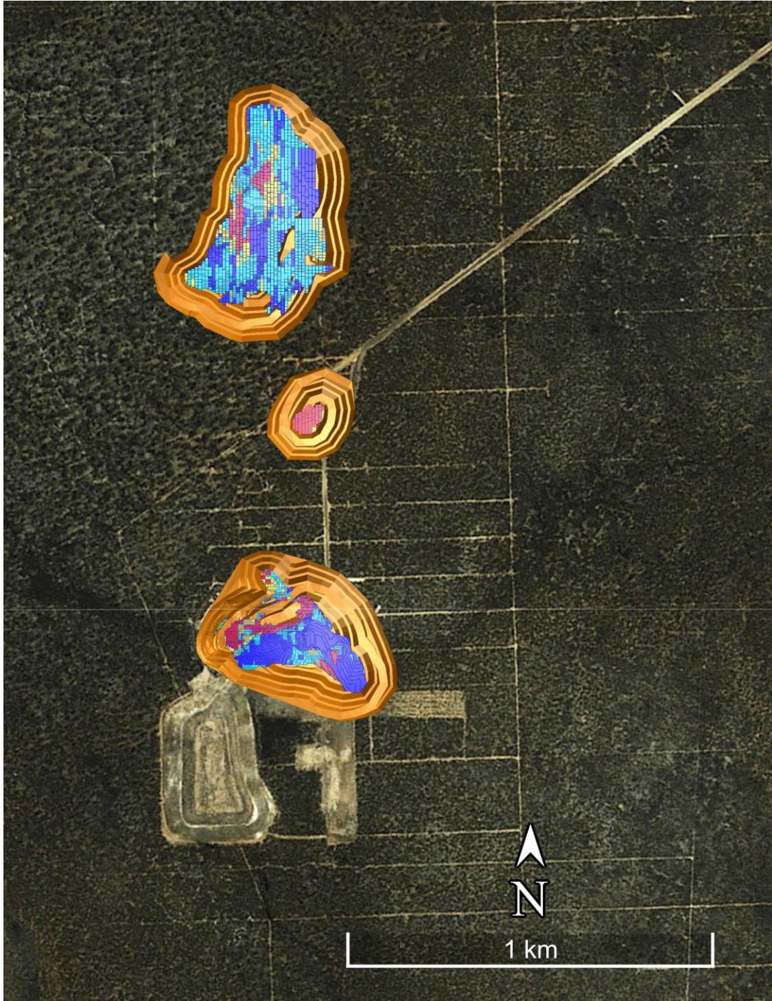
Figure 2 –Optimised Pit Shells as Designed by Auralia overlain on google earth Figure 2 –Optimised Pit Shells as Designed by Auralia overlain on google earth, colour grading index for blocks shown in Figures 3 & 4
