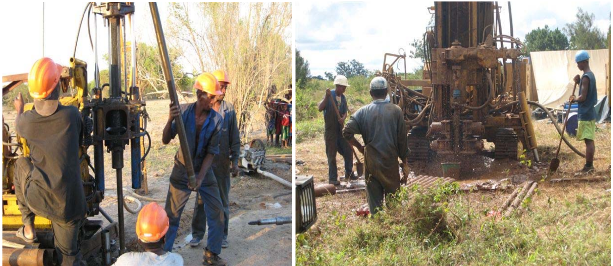
Long Year 34 Core rig (left) & Atlas Copco B-31 RAB rig (right) at work in the field
