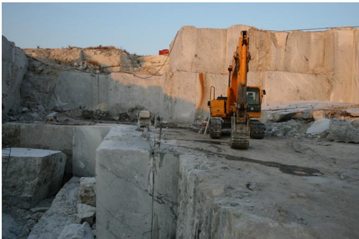
Labradorite blocks being cut using a cable ('Gang') saw (center of picture to left of excavator) - Magrama-lanapera. The saw operates on a rotating loop of cable and can take up to 8 hours to complete a cut.
