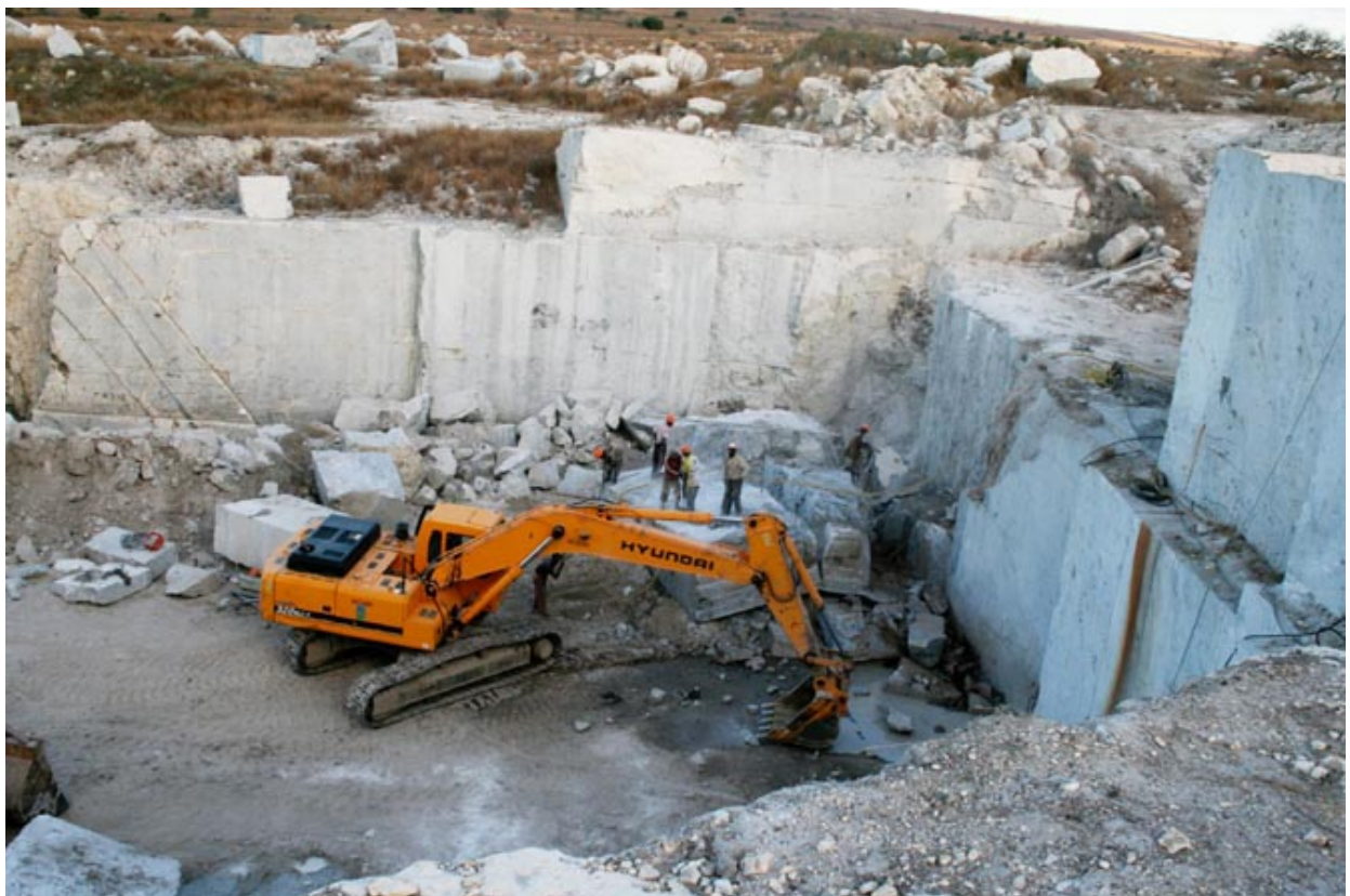
Excavator being used to clear access for cutting new blocks – Magrama-lanapera quarry
