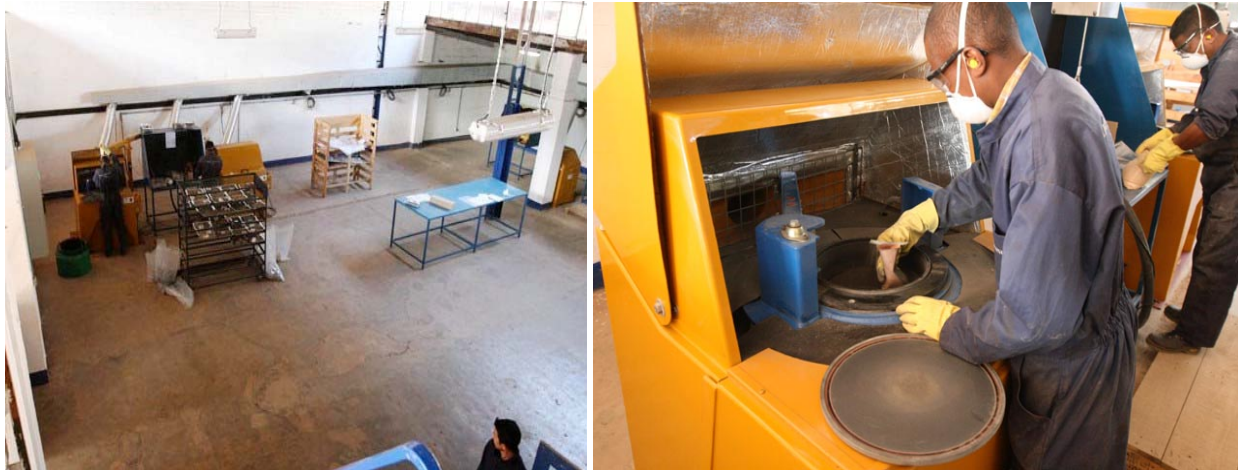
Left: GLS-ITTK facility processing samples; Right: Close-up of LM-5 pulverisers in operation
