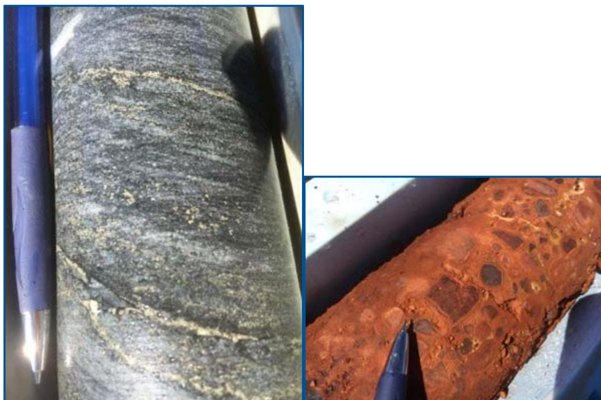
Figure 11: Mineralised Laterite and Fresh, sulphidic drill core from Bibra deposit, September 2016
