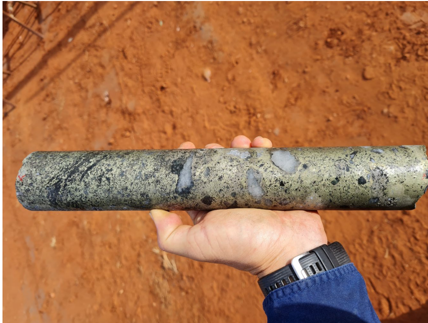
Figure 2. Photo of breccia copper mineralisation from NLDD042.
