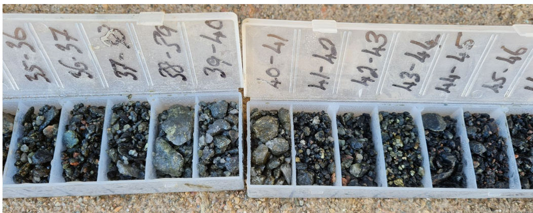
Figure 3. Lady Fanny RC drill chips from LFRC013.
