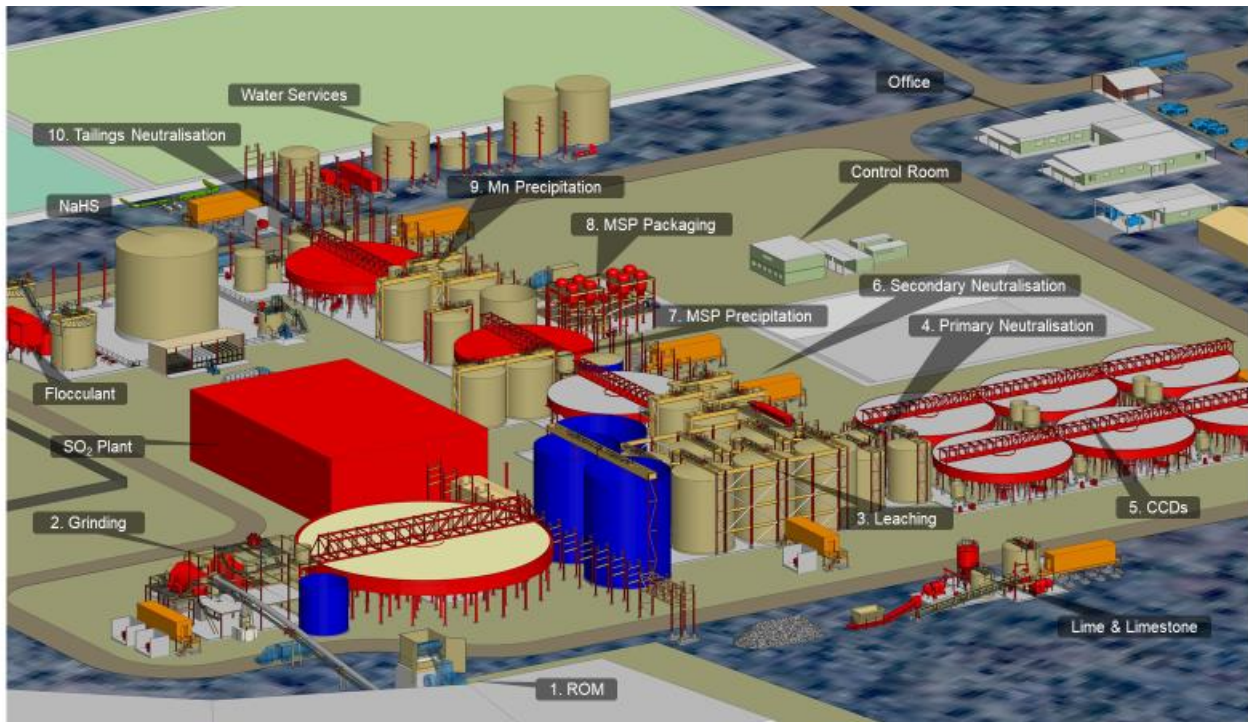
Figure 17 - 3D isometric of the Mt Thirsty processing plant showing generalised process flow (numbered labels)
