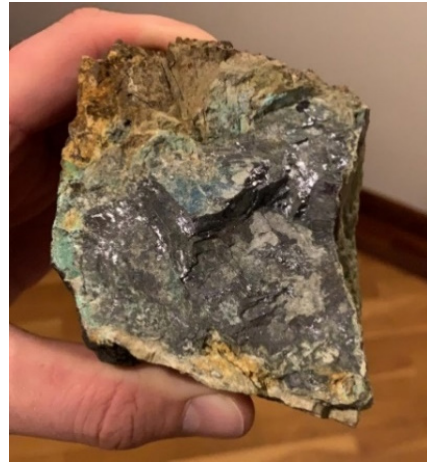
Figure 5: Mestersvig Project, rock chip sample 4958 showing massive galena hosted in a quartz vein.
