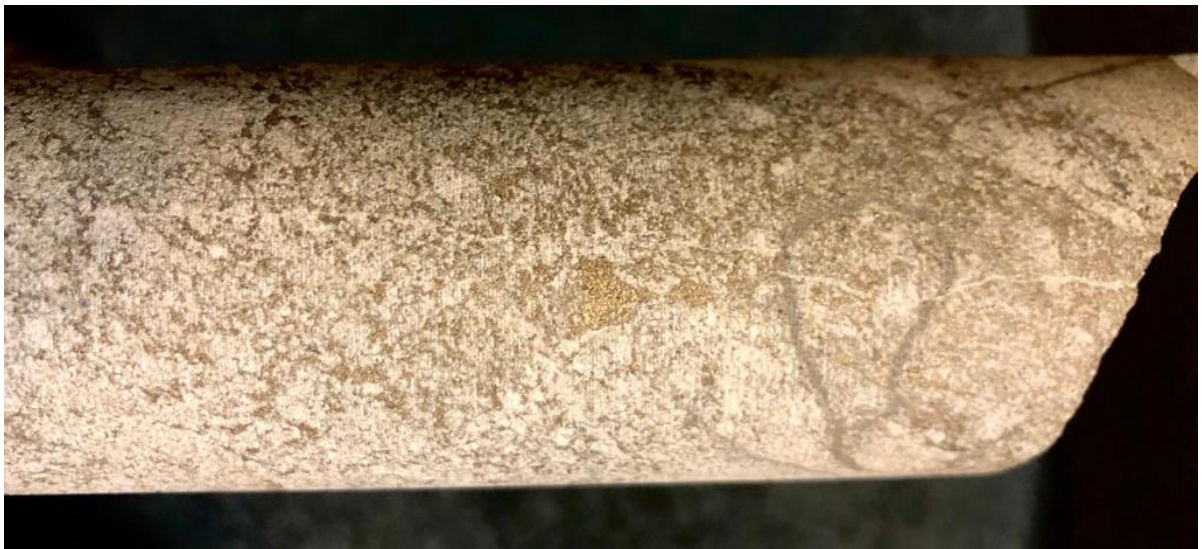
Figure: 2 Sulphide mineralisation in drill-hole MIDD003 from 97.31 to 97.43m downhole.
