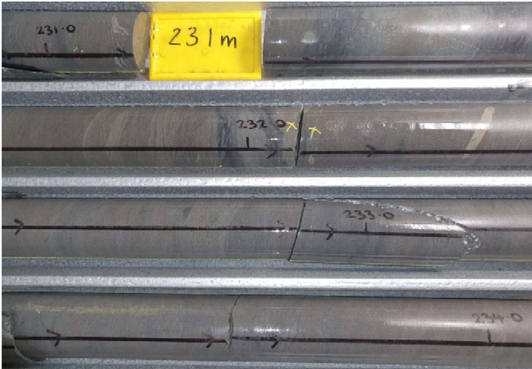
Figure 5: Lenses of sulphide mineralisation commencing at 230.9m downhole in CADD001.
