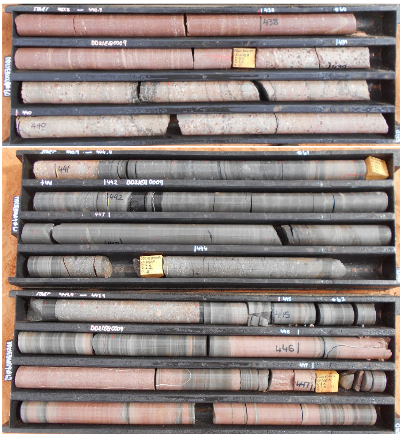
Figure 5 Core photos showing the mineralised intersections in hole DD21EB0009. Note the pink sandstone and grey breccia interbeds at the lower contact which are lower in Cu and are the primary cause of the internal dilution.
