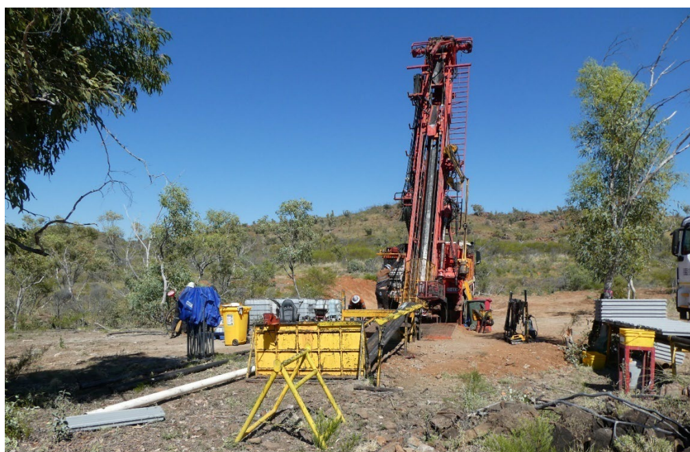
Plate 4: Diamond Drilling in Progress at King Solomon 1
