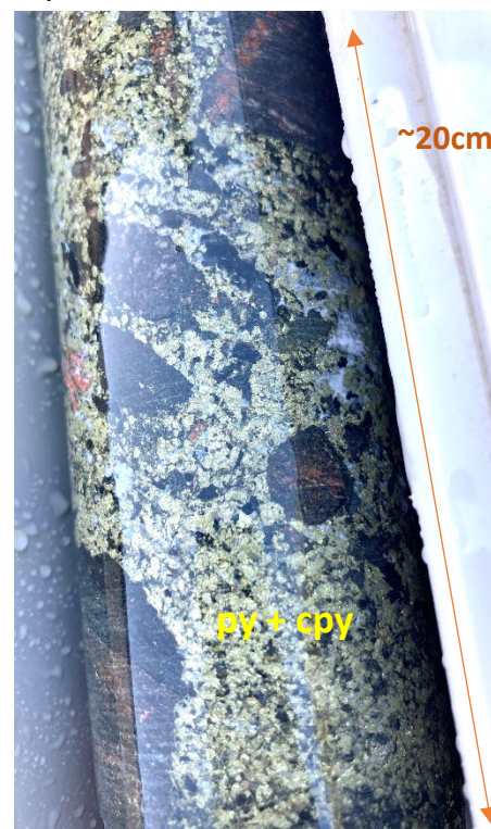
Plate 2: drill core from hole 22MEDH002, from ~ 87.5m downhole, semi massive sulphides in breccia
