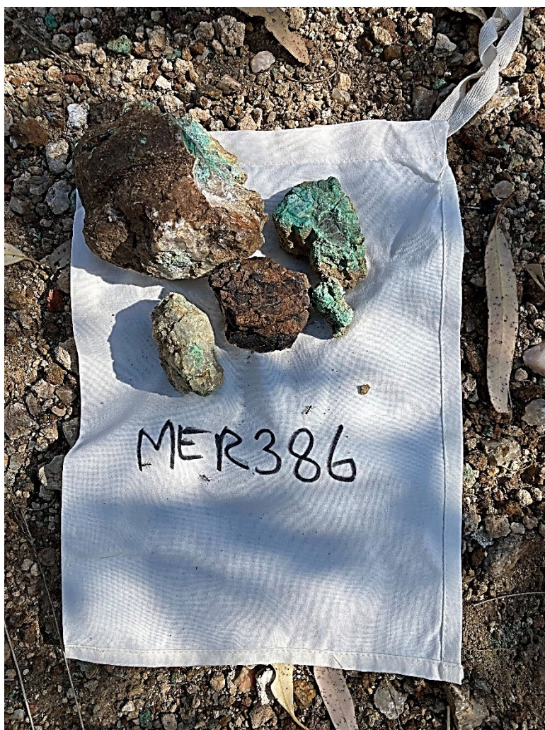
Plate 1: Rock chip (MER386) with 52.8g/t Au and 12.35% Cu
