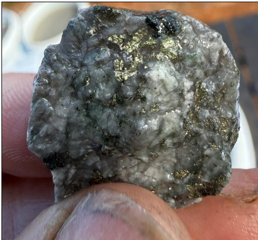
Figure 3 Chalcopryrite with interpreted magnetite in a quartz-rich RC chip, Ardmore North [hole 26MIE-005, @ 22-23m]. Visual identification only; not confirmed by assay and not indicative of grade or width. Image unedited; fingers for scale.
