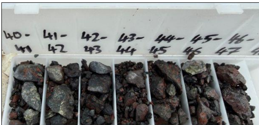
Figure 1 Representative example of sulphides (chalcopyrite \pm pyrite) visually identified in RC drill chips. [Hole 26MIE-011, @ 40-47m m downhole; Ardmore North.] Image unedited; colours not enhanced; Downhole depths annotated on tray are in metres. Visual identification only; not confirmed by assay and not indicative of grade, width or continuity. Depth range shown is the extent of the chip tray photographed; sulphides occur at points within it, not as a continuous interval.
