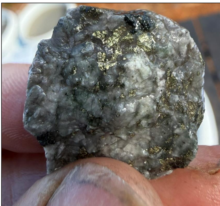
Figure 3 Chalcopyrite with interpreted magnetite in a quartz-rich RC chip, Ardmore North [hole 26MIE-005, @ 22-23m]. Visual identification only; not confirmed by assay and not indicative of grade or width. Image unedited; fingers for scale.
