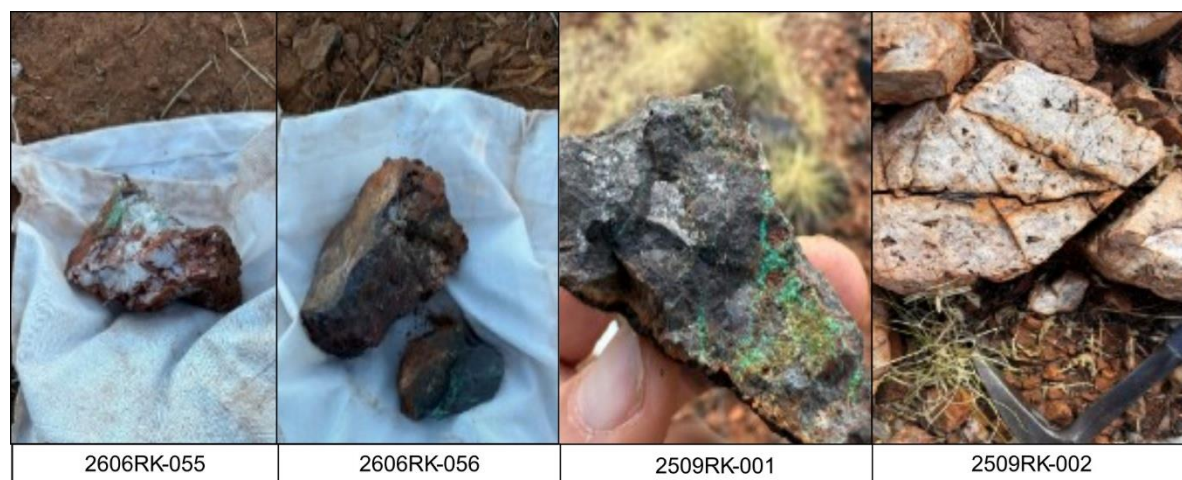
Figure 1: Rock Chip Samples 2606RK-055 and 2606RK-056 from RC drill pad. 2606RK-055 quartz vein with malachite on fractures. 2606RK-056 is a hematite-magnetite ironstone with malachite. 2509RK-001 Hematite magnetite gossan. Malachite and sulphides (pyrite & chalcopyrite). 2509RK-002 Quartz feldspar breccia with boxwork textures and anastomosing quartz veins.
