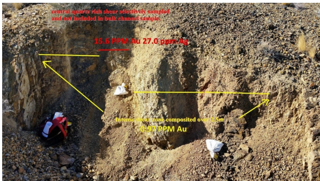
Figure 9: Bulk Channel Sampling & assay locations Lambarson Canyon, a potential high-grade Carlin Type system with similar Geological setting to the 4.0 M ounce Lone Tree deposit:
