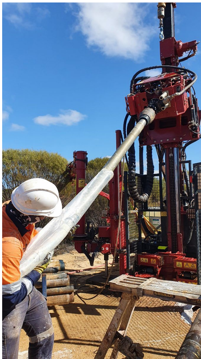
Figure 1: Drilling bright white kaolin at Tampu Kaolin Project, Beacon WA
