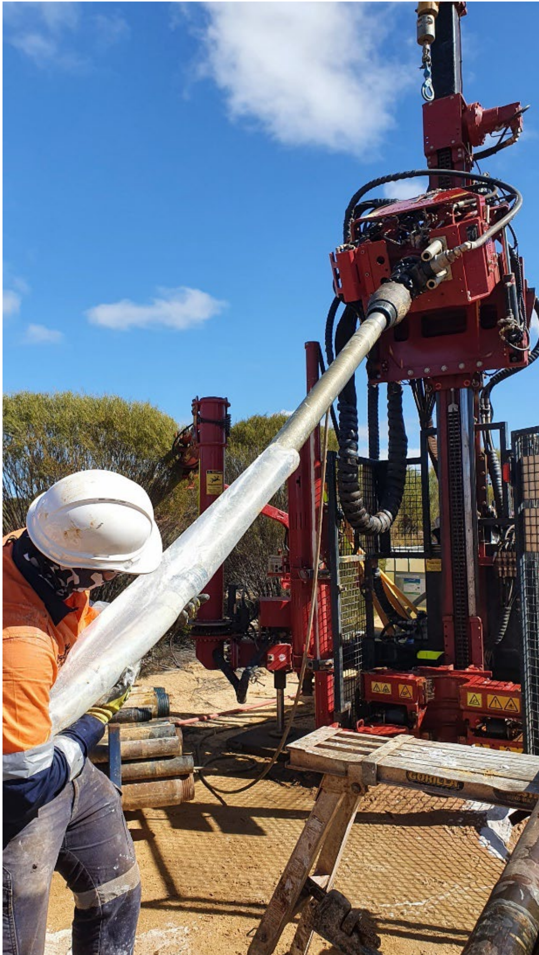
Figure 5: 2022 Resource Definition Sonic drilling at Tampu
