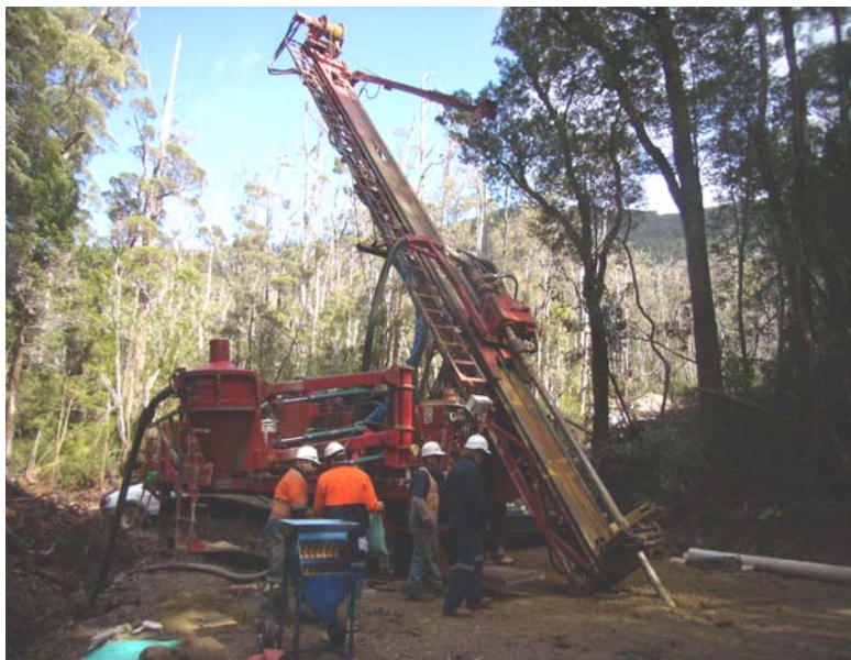
Multipurpose Drill Rig drilling the first Reverse Circulation drill hole at Stanley River
