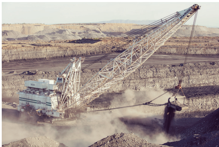
Above Dragline 303 in operation at Curragh
