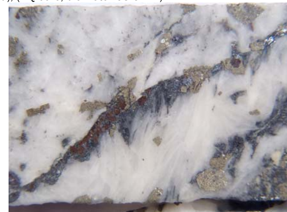
Figure 10: SGRDD004, 58.3 metres. 19.6 grams/tonne gold from 58-59 metres downhole including 2.18 ounces/tonne silver and 0.64%/tonne antimony (HQ core, diameter 63.5mm). Vein filling composed of abundant medium to coarse grained carbonate (calcite), plus crudely banded and disseminated medium to coarse grained sulphides, minor, but locally abundant fine-grained sericite and a little quartz. Pyrite is the most abundant sulphide mineral, and together with subordinate arsenopyrite, is paragenetically early. There was subsequent deposition of sphalerite, galena and stibnite, with local evidence of replacement of pyrite and arsenopyrite. Stibnite is commonly associated with galena, and has possibly replaced the latter. A trace of fine grained chalcopyrite occurs with sphalerite and also hosted in carbonate (field of view 50mm).
