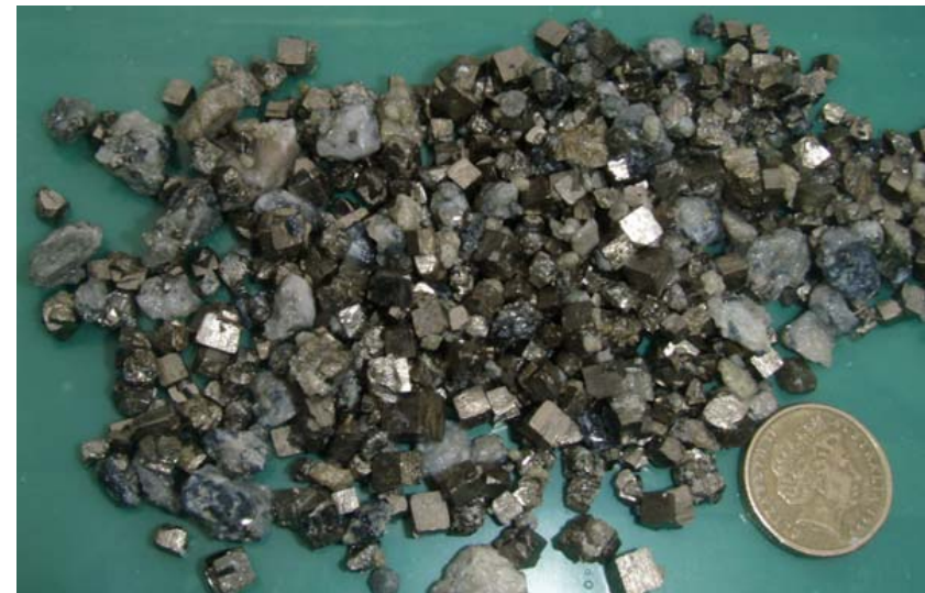
Figure 14: SGRRC017, euhedral pyrite and arsenopyrite, 86-89m.
