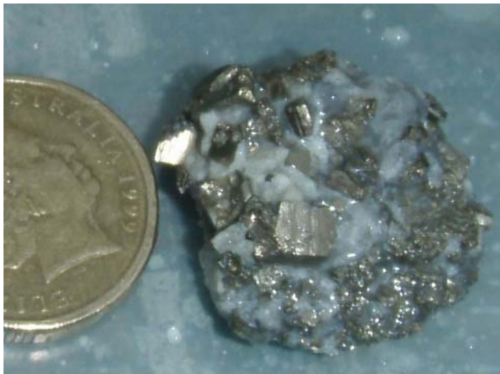
Figure 13: SGRRC0011, euhedral pyrite, 1.53 grams/tonne gold, 60-61m.
