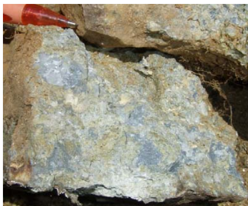
Frasers Find – Sample FFSB – High grade quartz-sulphide (abundant arsenopyrite, pyrite, galena) from the dump by the main shaft, assayed 76.9 g/t gold (2.47 ounces), 287 g/t silver (9.23 ounces) and 1.78% lead/tonne (ALS Certificate of Analysis BR12004879).
