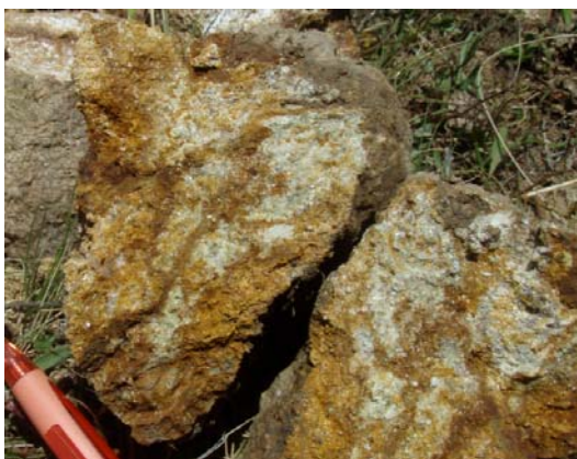
Frasers Find – Sample FF3D – Disseminated mineralisation in altered granite adjacent to main high-grade lode. Quartz-sericite altered granite with disseminated sulphides (much now oxidised to yellow limonite) and sheeted quartz-sulphide veins. Assayed 3.43 g/t gold and 5.91 g/t silver (ALS Certificate of Analysis BR12004879). Drilling is planned to test the width of the disseminated mineralisation, the high-grade lode and for repetitions of high-grade parallel veins.
