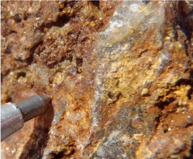
SGRDD023: Quartz-iron oxide (after sulphide) mineralisation. 19.1g/t Au (14.25g/t Au duplicate), 141g/t Ag and 0.75% Pb over 0.6 metres (~40% length recovery from 11.1-11.7 metres downhole)
