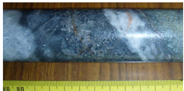
SGRDD030: IRGS sheeted quartz-sulphide veins in altered granite. 1.17g/t Au over 0.82m including a narrow high grade sulphide portion of 5.64g/t Au (4.08g/t Au duplicate) over 0.08 metres (from 38.26 - 39.08m downhole)
