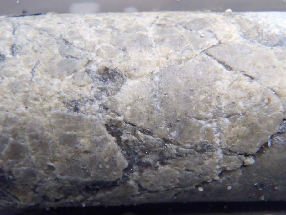
SGRDD038 , 41.7m, Martins Shaft-style alteration. Extensively altered felsic dyke exhibiting brecciation, phyllic alteration and disseminated and fracture hosted sulphides.
