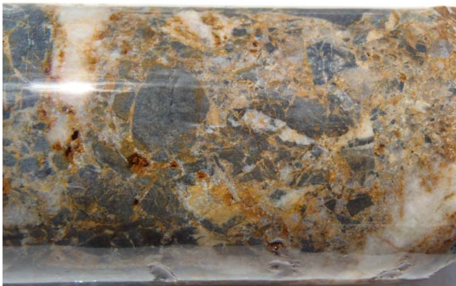
SGRDD036 , Core of Sample D3609B, 3.28 g/t Au. Intensely altered (silica-sulphide) and brecciated metasediments.
