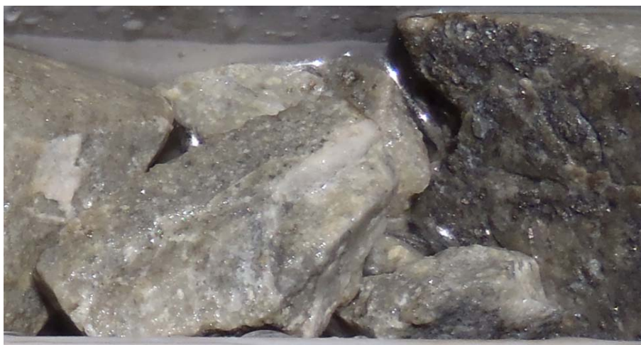
SGRDD038 , Core of Sample D3841, 1.93 g/t Au. Extensively altered felsic dyke exhibiting brecciation, phyllic alteration and disseminated and fracture hosted sulphides.
