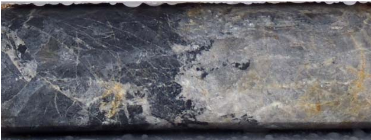
SGRDD036 , Core of Sample D3609A, 12.35 g/t Au. Intensely altered (silica-sulphide) and brecciated metasediments.
