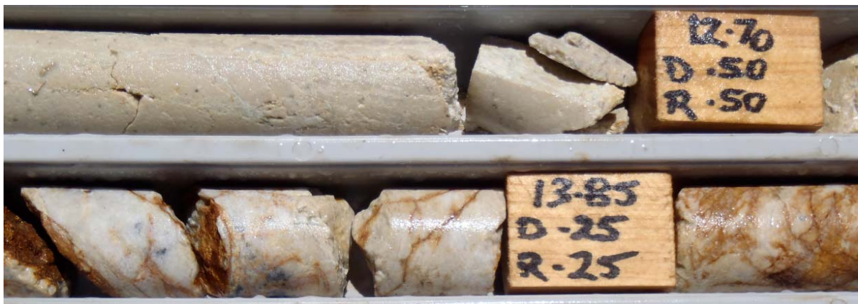
SGRDD039 , Core of Samples D3913, 2.05 g/t Au (top row of core tray) and D3914B 1.31 g/t Au, 453 g/t Ag and 0.14% Sb (stibnite, antimony oxide) bottom row of core tray. Extensively altered felsic dyke exhibiting phyllic alteration, some brecciation and disseminated and fracture hosted sulphides.
