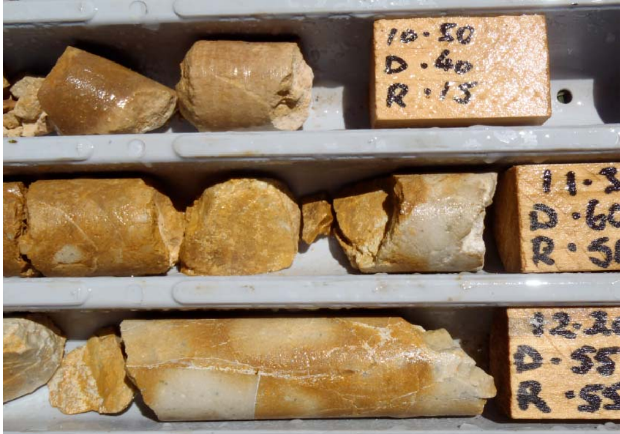
SGRDD039 , Core of Sample D3911B, 4.93 g/t Au (middle row of core tray) and D3912B, 1.90 g/t Au (bottom row of core tray). Intensely altered felsic dyke exhibiting phyllic alteration, fracturing/brecciation and disseminated and fracture hosted sulphides.
