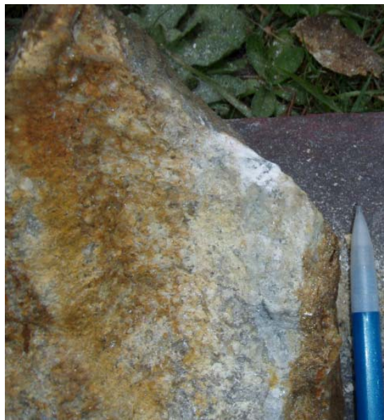
Melvaines Mine, Sample S415, 1.3 grams/tonne Gold. Disseminated quartz-sulphide alteration associated with closed-spaced narrow sheeted veins.
