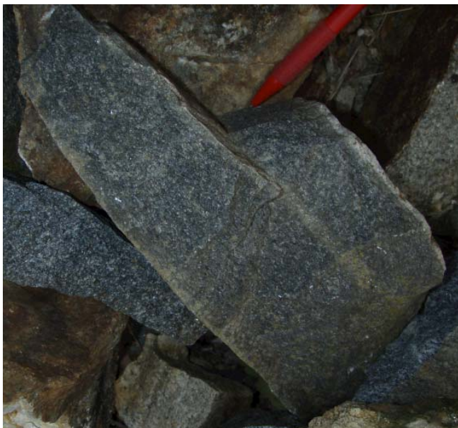
Melvaines Mine, Sample MM1, 2.12 grams/tonne Gold. Narrow sheeted quartz-sulphide veins (light coloured linear structures) in altered dyke like those drilled at Martins Shaft.
