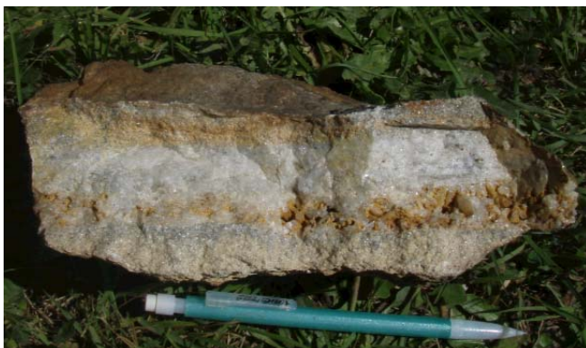
Melvaines Mine, Sample MM2, 0.64 grams/tonne Gold, 2cm wide sheeted quartz-sulphide vein in quartz-sericite altered dyke. Limonite staining after sulphides in vugs associated with prismatic quartz. This open texture of this sample exhibits a high level epizonal (epithermal equivalent) IRGS setting that indicate the bulk of the system is preserved at depth.
