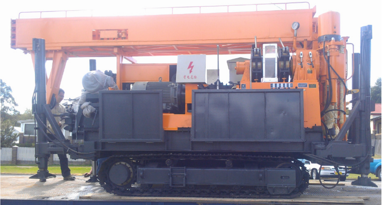
Track mounted deep drilling (600 metres) diamond drill rig. This rig has a very low environmental footprint as it is able to crawl to drill site and level itself with hydraulic jack legs, therefore it does not need the support of earthworks such as roads and drill pads.
